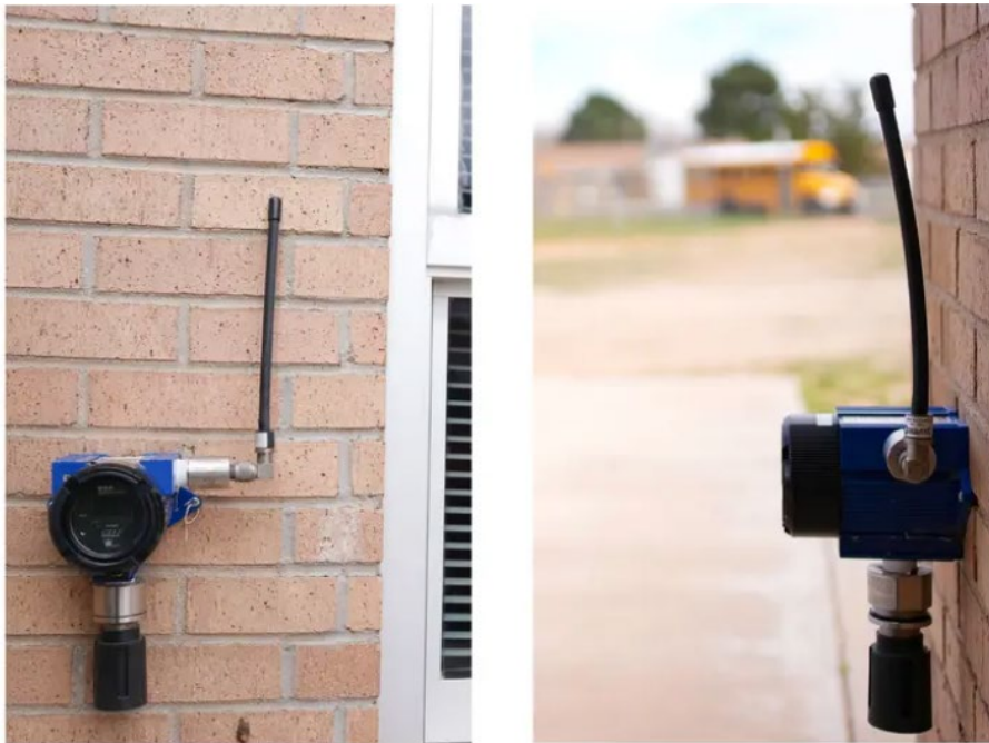
Air monitors to detect hydrogen sulfide outside of Noel Elementary School in Odessa on March 6, 2024. The system doesn't log the H 2 S concentrations it detects.
